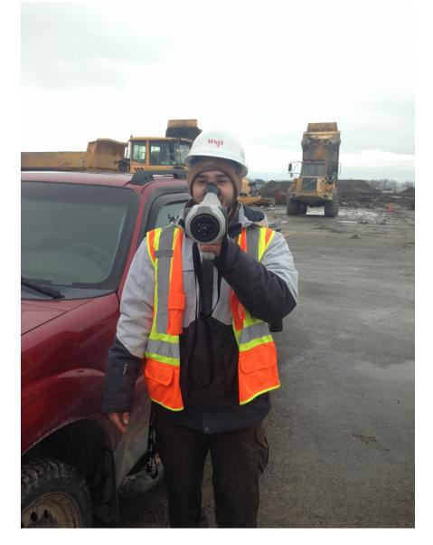
We use a nasal ranger or olfactometer to measure existing odour in and around the construction site.
